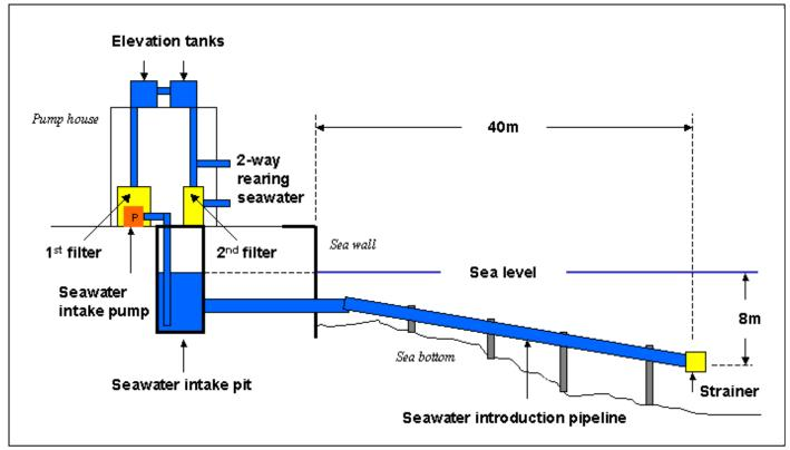
2-1 Lateral view of water intake system of VFD's hatchery
