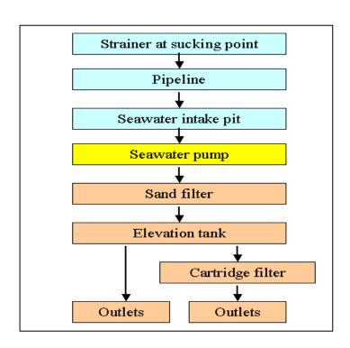
2-2 Diagram of seawater intake system
